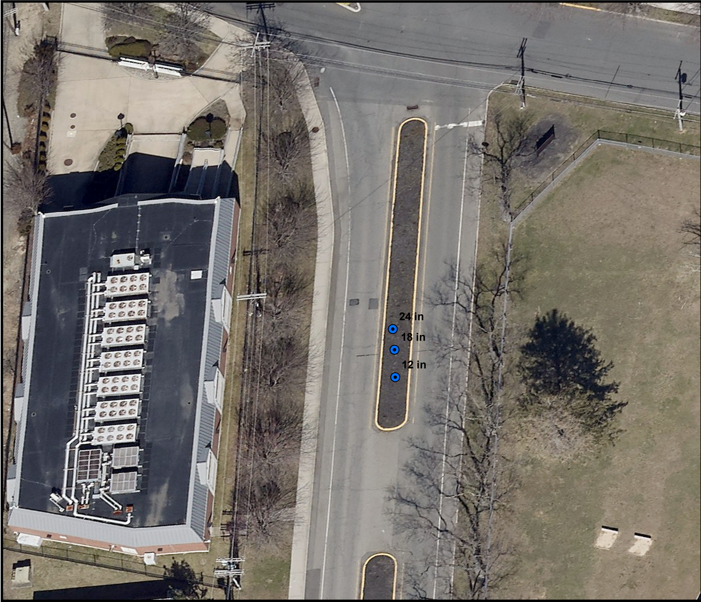
Figure SG3 Rain Garden Percolation Test Sea Girt National Guard Training Center
